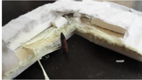
Figure 7: Cohesion of non impacted and remaining glued ceramic tiles on the final target
