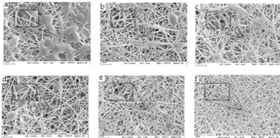
**Figure 1.** Scanning electron micrographs of neat PU and PU/MWCNTs electrospun nanofibers at applied voltage of 10 kV . MWCNTs content was (a) 0% wt.%, (neat PU) (b) 2% wt.%, (c) 4% wt.%, (d) 6% wt.%, (e) 8% wt.% and (f) 12%.
