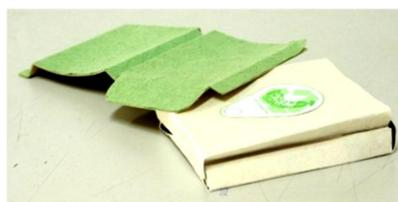
**Figure 1:** green packaging from banana fiber for instant food products as envelope style (Stand-up pouch)
